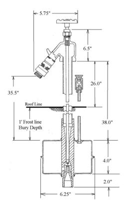
Roof hydrant shall be the Freeze Flow Roof Hydrant Model # 2131R manufactured by Hoeptner Perfected Products, Gilroy, CA.
