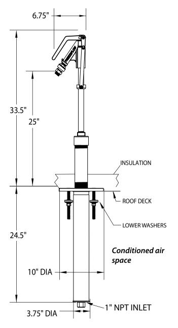
Roof hydrant shall be the Freeze Executive Flow Roof Hydrant Model # 2131RE manufactured by Hoeptner Perfected Products, Gilroy, CA. 408-847-7615
