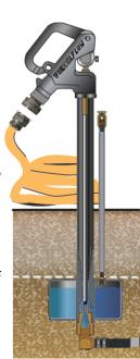
Empty the reservoir by operating the hydrant at full flow for 30 seconds to
