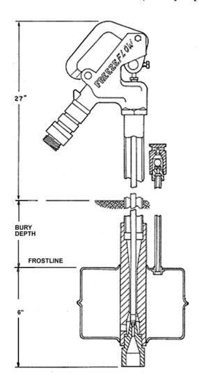
Sanitary Yard Hydrant shall be the Freezeflow Standard ADA/ Lever Model # 213XADA ( X represents bury depth, i.e. 2134ADA – 4' bury) manufactured by Hoeptner Perfected Products, Gilroy, CA
